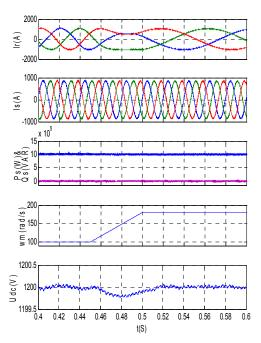
Figure 5. Responses Rotor and Stator Current, Active and Reactive Power, DC Link Voltage with Rotor Speed Varying from 100 rad/s to 180 rad/s
