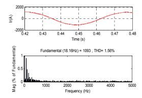
Figure 6. Harmonic Spectrum of Stator Current
