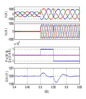
Figure 3. Responses Rotor and Stator Current, Active and Reactive Power, DC Link Voltage ( $w_m$ = 100rad/s)
