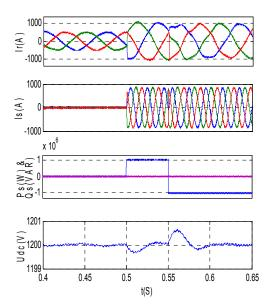
Figure 4. Responses Rotor and Stator Current, Active and Reactive Power, DC Link Voltage (wm= 200rad/s)
