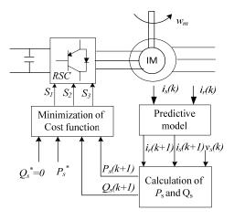
Figure 2. Schematic of the Original Predictive DPC Control Strategy of Rotor Side PWM Converter
